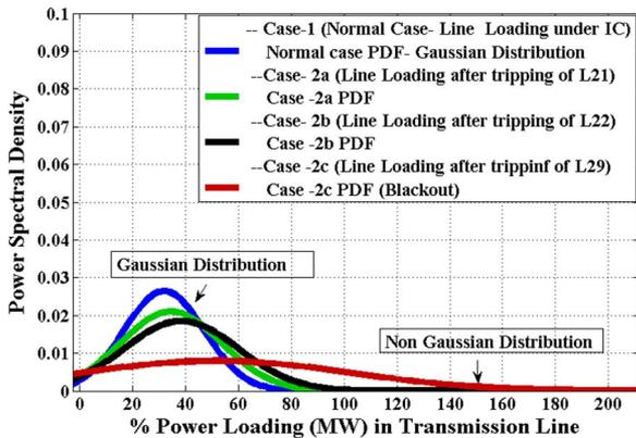
Fig. 12. Gaussian to non-Gaussian distribution of power in the test-bed system.
