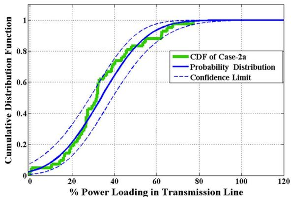
Fig. 7. Case 2a: CDF plot after tripping of line L21.
