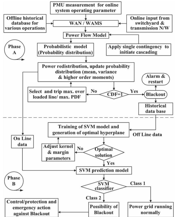
Fig. 1. Proposed model for proactive cascade failure prediction.
