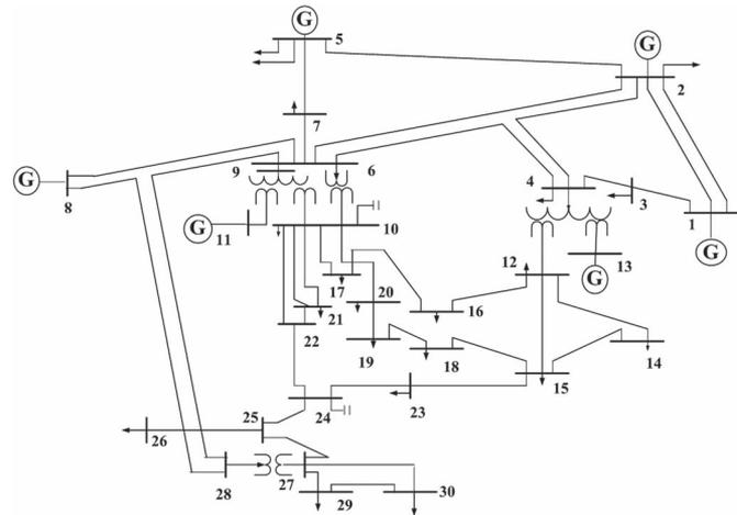
Fig. 2. One-line diagram of the IEEE 30-bus test-bed system.
