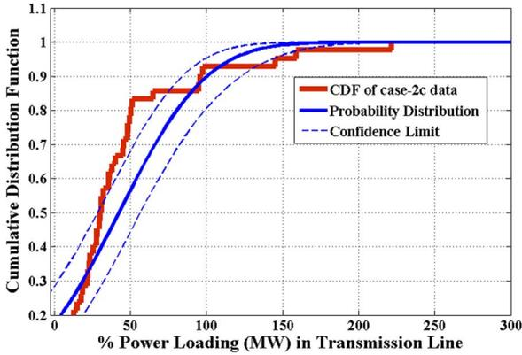
Fig. 11. Case 2c: CDF plot after tripping of line L29.
