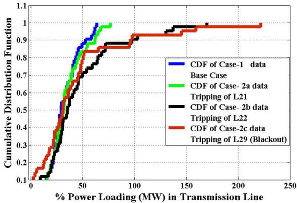
Fig. 13. CDF plots of normal to blackout cases in the IEEE 30-bus test-bed system.
