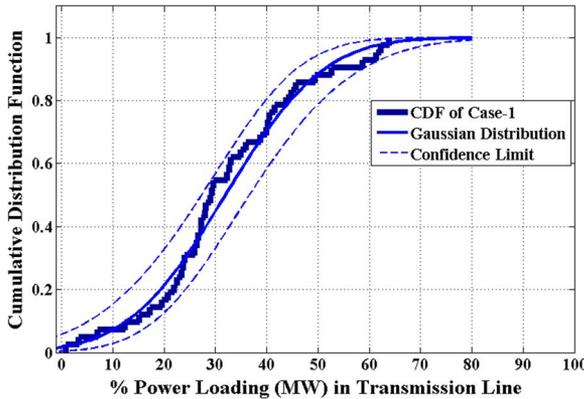
Fig. 5. CDF plot as a function of power flow in the transmission line.
