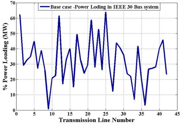
Fig. 3. Power flow in transmission line of test-bed base case.
