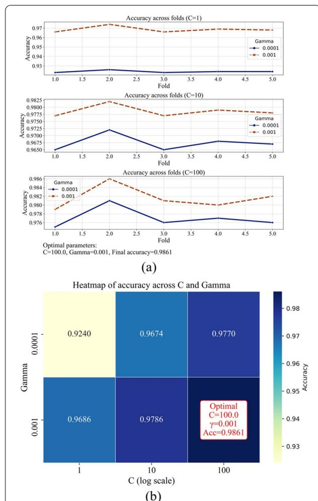
**Fig. 2** SVM parameter tuning and identification of optimal parameters for maximum performance. **a** Accuracy across folds for different values of C and gamma, illustrating the model’s performance consistency during cross-validation, **b** heatmap showing the mean accuracy across combinations of ‘C’ and ‘gamma’, highlighting the optimal parameters (C = 100, gamma = 0.001) with the highest accuracy of 0.9861
