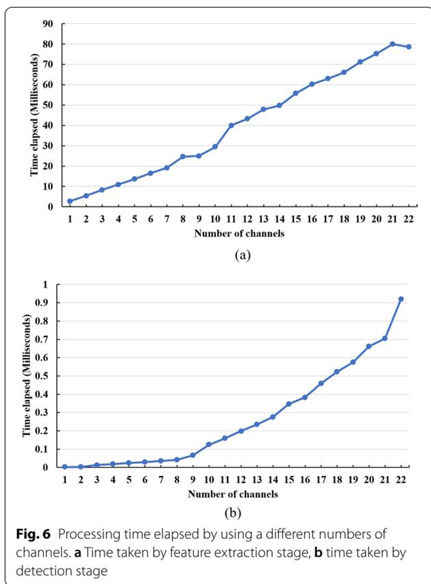
**Fig. 6** Processing time elapsed by using a different number of channels. **a** Time taken by feature extraction stage, **b** time taken by detection stage
