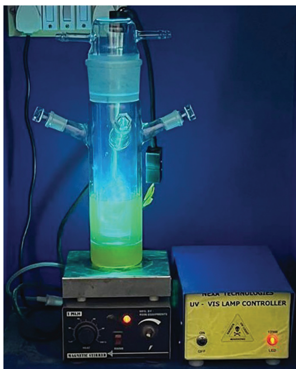
Fig. 4. Photodegradation reaction performed in the presence of catalysts (medium-pressure mercury UV lamp, UV light range (250–400 nm)).
