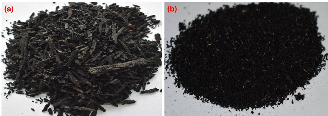
Fig. 1 a Uneven raw Waste tire rubber b waste tire rubber powder (Grain size—425 \mu\text{m} )
